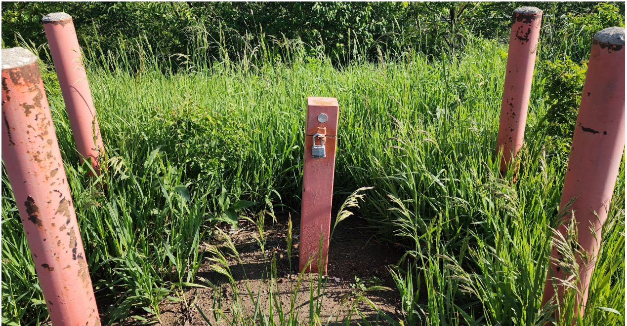
Photo 9 Monitoring well MW-102. Typical monitoring well configuration with bumper posts. May 29, 2025.
