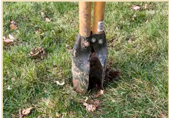
Using a clamshell posthole digger to create a hole for the perc test.
