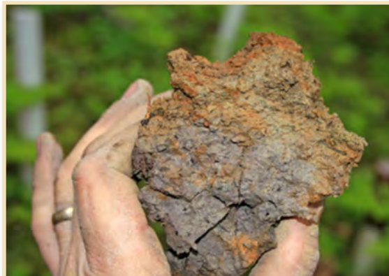
Gray color indicating high levels of moisture in the soil.
