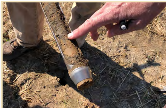
Accessing subsoils using a soil probe.
