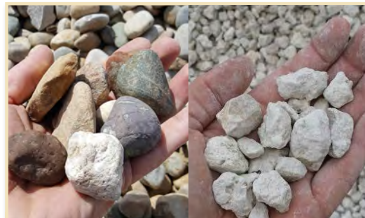
1-inch washed field rock and crushed limestone rock.
