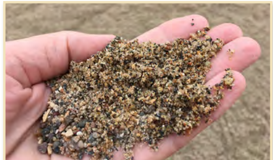
Concrete sand is added to rain gardens to enhance percolation.
