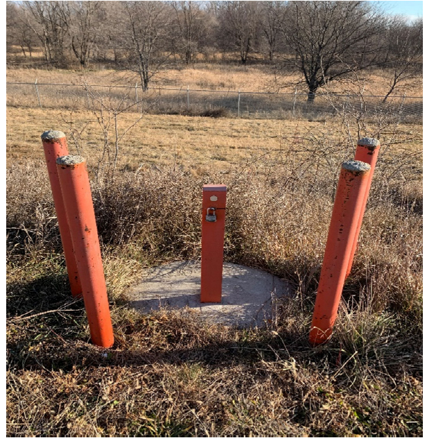
Photo 26: 2021 Typical groundwater monitoring well installed in June 2018.
