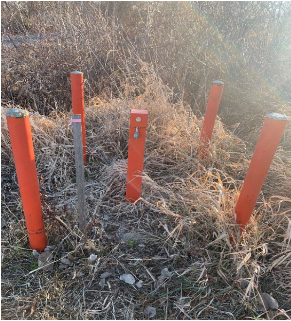
Photo 25: 2020 Typical groundwater monitoring well installed in June 2018.
