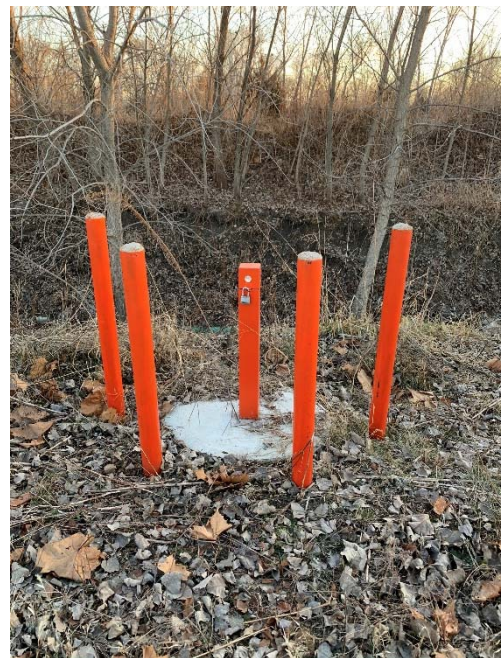
Photo 28: 2019 Typical groundwater monitoring well installed in June 2018.
